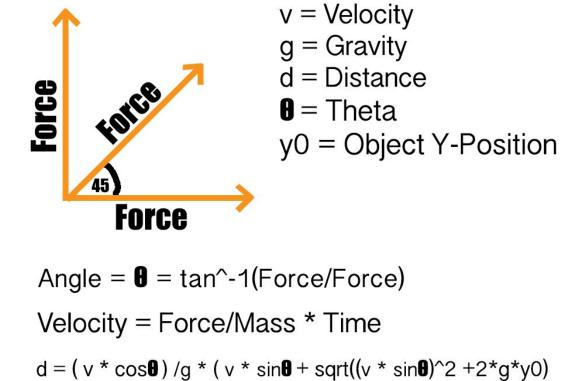
When we get the force that is being applied on the Y-axis and Z-axis of the object we can figure out the angle it will be launched at. As you can see in the figure above, the angle equation is how we figure out the angle it will be launched at. By knowing the angle it is launched at, the velocity of the object, and its y position we can plug it all into the distance equation, and be able
